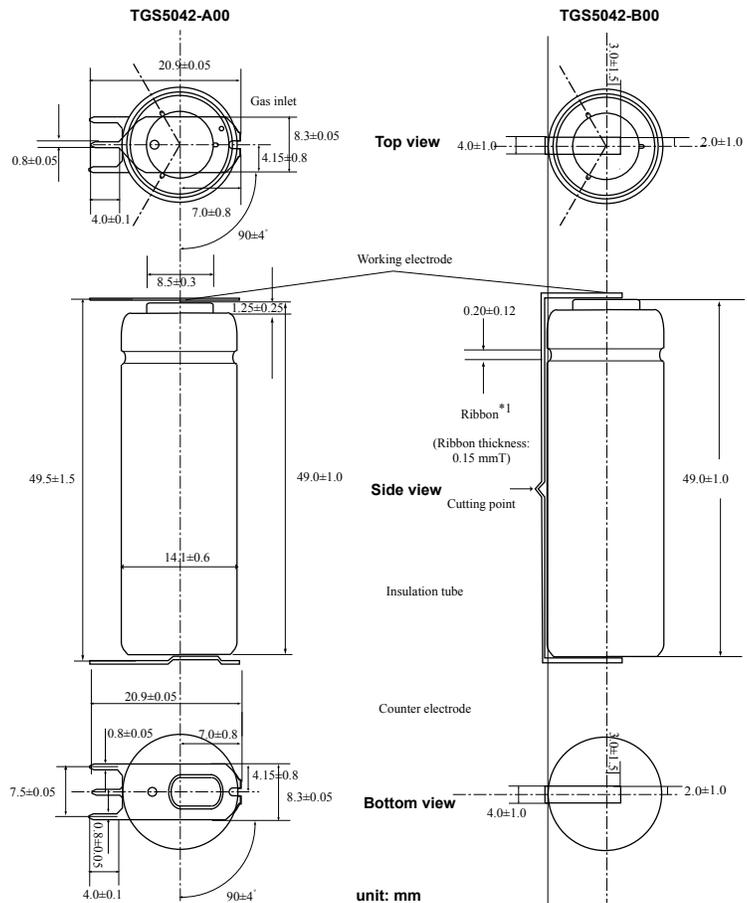
**NOTE 1:** When the sensor is shipped, the working electrode and counter electrode are connected (i.e. short circuited) by a spring (-A00) or a metal ribbon (-B00) in order to avoid polarization of the electrodes. To measure the sensor output, the spring should be removed (-A00) or the ribbon should be cut (-B00) and the sensor connected to a measuring circuit (see example above). The cutting point as indicated can be used to cut the ribbon easily.
