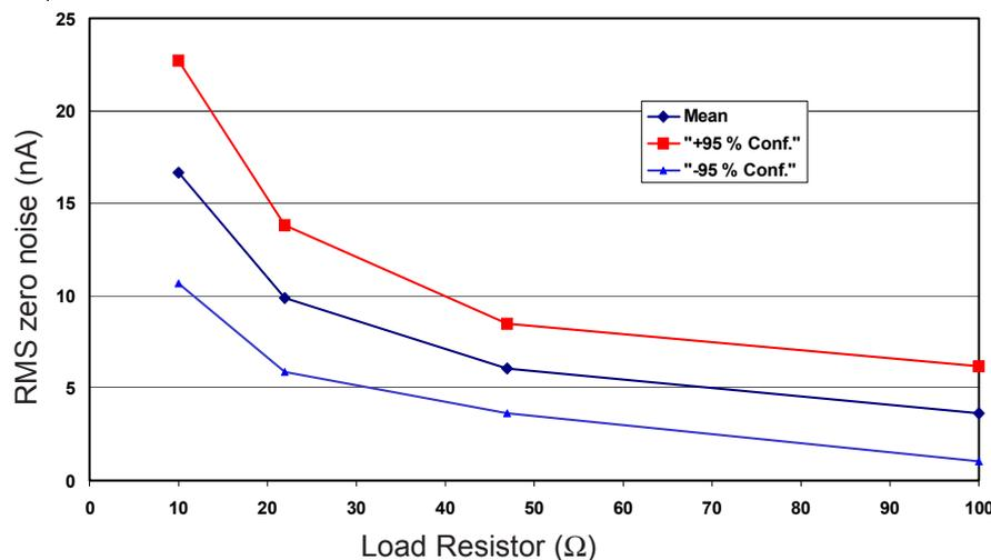
Figure 3 shows the effect of the load resistor on the RMS zero noise for the NO2-B1 sensor. The mean and  $\pm 95\%$  confidence intervals are shown.
