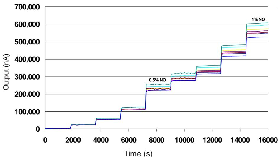
The NO-AE shows fast, stable response from 0 to 1% NO.
