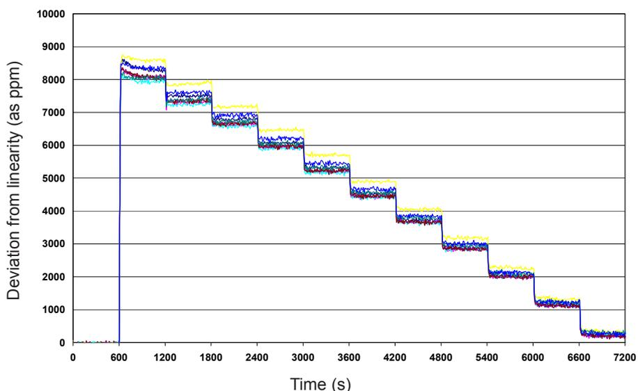
Eight PH3-B1 were tested for response from 10 to 1ppm.
