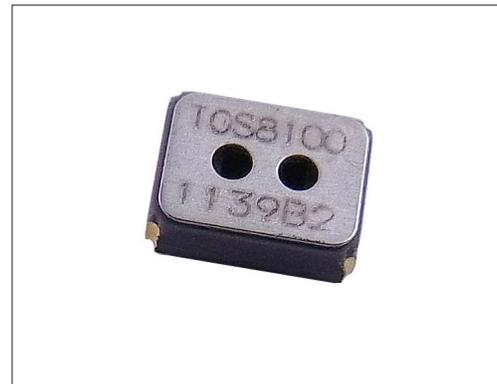
The **TGS 8100** has high sensitivity to low concentrations of gaseous air contaminants such as cigarette smoke and cooking odors. By utilizing the change ratio of sensor resistance from the resistance in clean air as relative response, human perception of air contaminants can be simulated and practical air quality control can be achieved.
