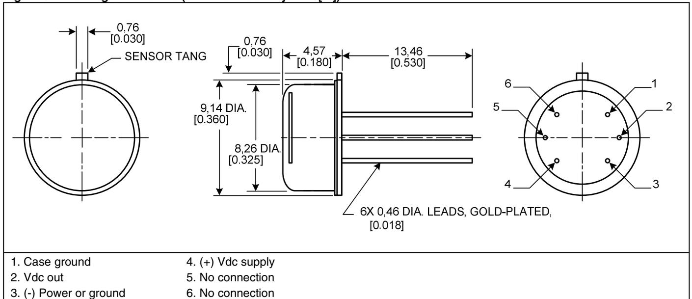
**Figure 6. RH Sensor Construction**
