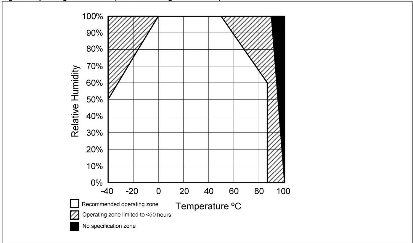
Figure 2. Storage Environment (Non-condensing environment.)
