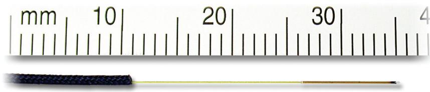
The FOS-N is a fiber optic strain sensor, ideal for composite material engineering research and civil-engineering applications such as structural health monitoring of buildings, bridges, tunnel linings and supports.
