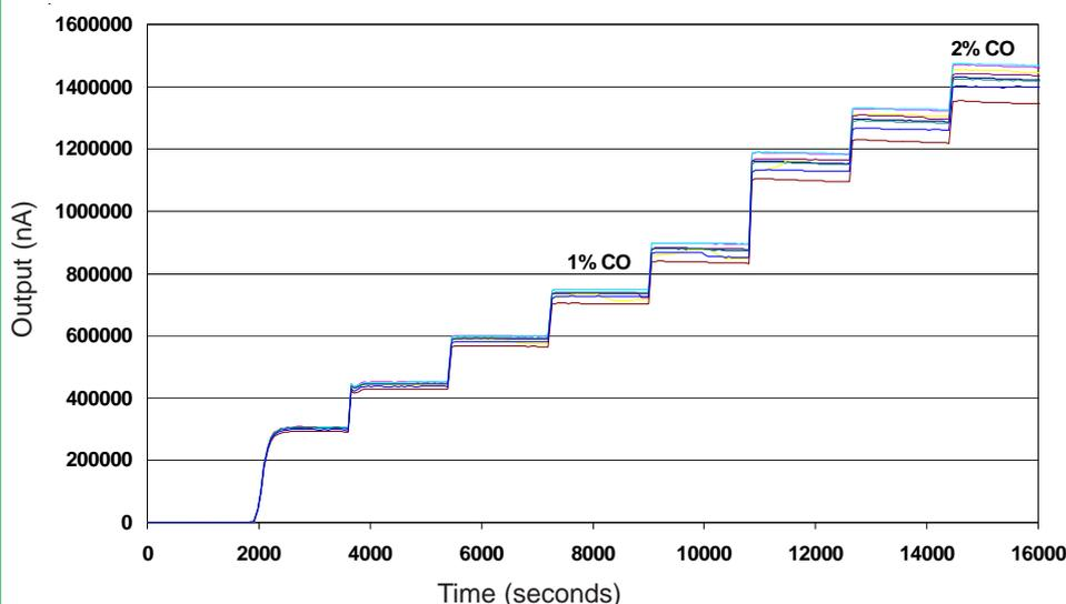
Figure 4 shows the excellent response to step changes in CO concentrations from zero to 2% CO by volume.
