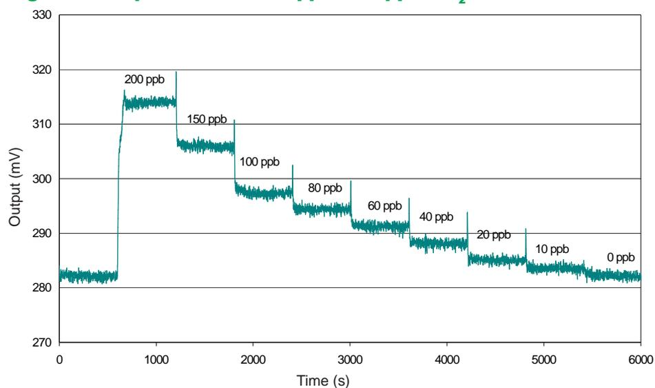
Figure 4 shows response from from 200ppb NO<sub>2</sub> to 0ppb NO<sub>2</sub>.
