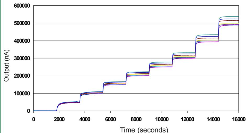
Sensor shows good response to 200ppm HCl.
