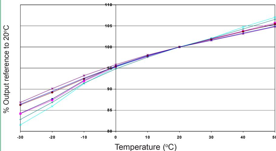
Figure 2 shows the variation of sensitivity at 25ppm HCl caused by changes in temperature.
