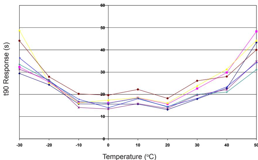
Figure 4 shows the response time temperature dependence for a typical batch of sensors.
