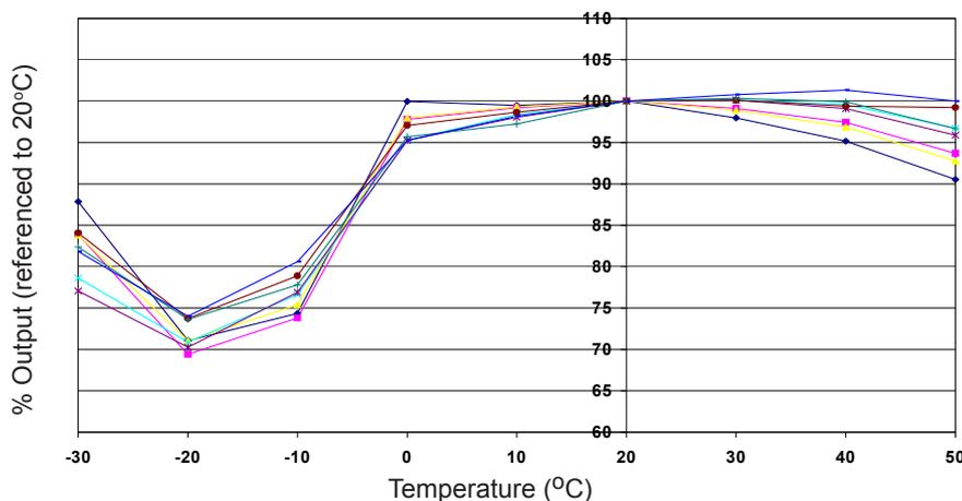
Figure 2 shows the variation in sensitivity caused by changes in temperature.
