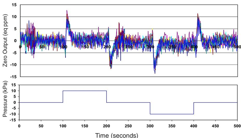
From ambient pressure, sensors were subjected to both positive and negative 10kPa pressure steps. The small transient rapidly decays as the sensor returns to its zero baseline.
