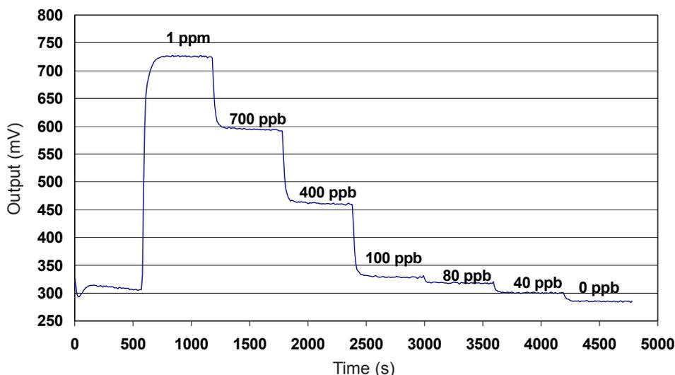
Figure 4 shows response from 0 to 1ppm CO.
