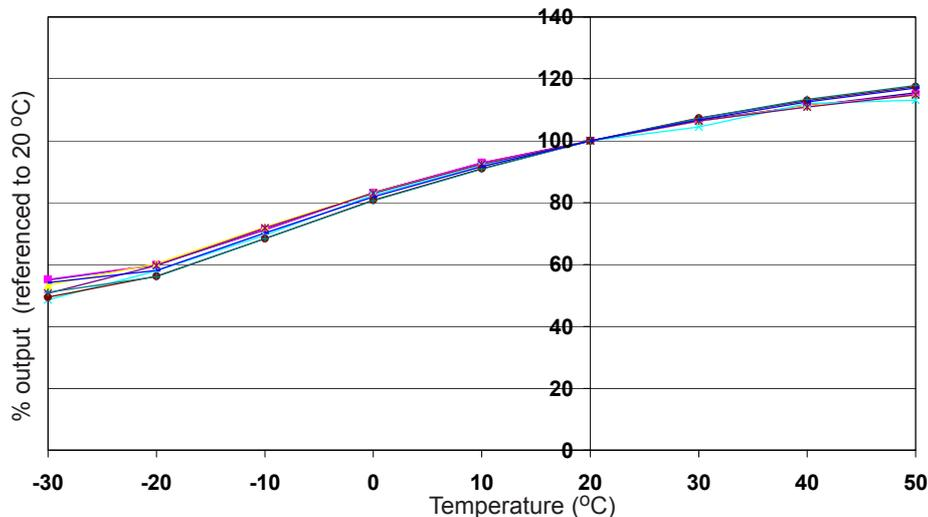
Figure 2 shows the temperature dependence of sensitivity at 2ppm CO.
