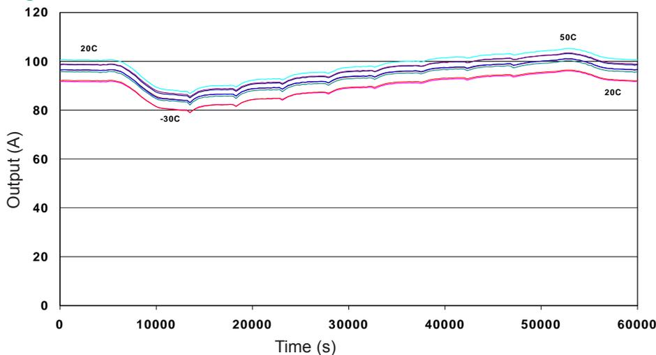
This time trace follows eight sensors' progress as they are first cooled to -30°C, then thermally stepped to +50°C before finally returning to 20°C.
