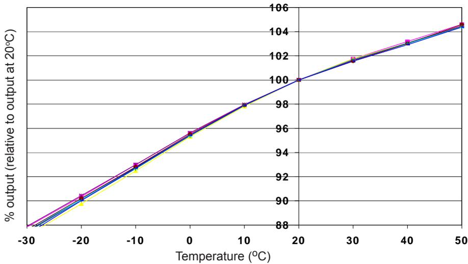
Figure 2 shows the very repeatable variation in sensitivity caused by changes in temperature.
