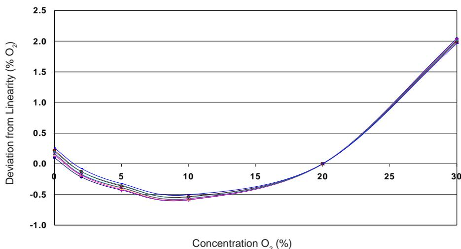
Mass flow oxygen sensors generate a non-linear current with increasing oxygen concentration:
