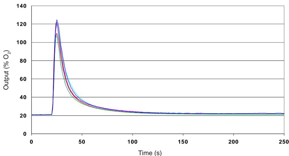
Step changes in pressure can cause a temporary signal transient. Positive pressure gives a output signal increase whilst negative pressure causes the output signal to decrease.
