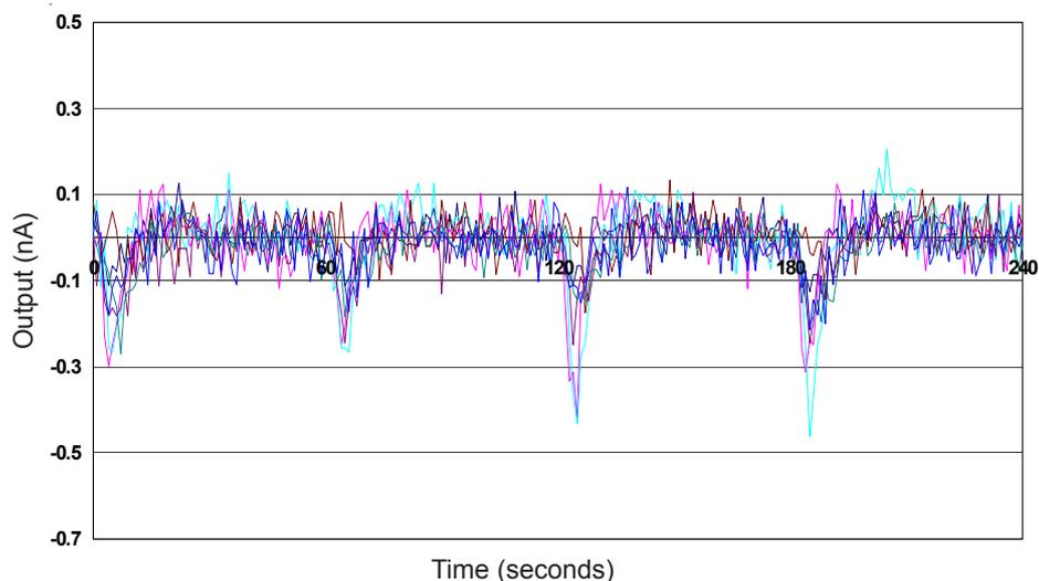
Figure 4 shows typical sensor outputs for a group of sensors exposed to exhaled breath for 4 cycles over 240 seconds.
