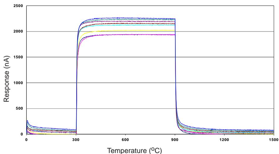
The HCN-A1 shows fast response and stable output when exposed to 30ppm HCN.
