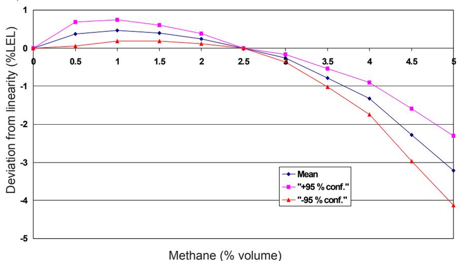
Figure 3 shows the non-linearity from 0 to 5% methane (volume). Sensor non-linearity at 100% LEL is less than 4%.
