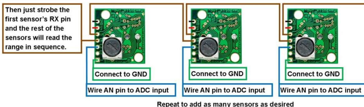
The next method is AN Output Constantly Looping. The first sensor will range, then trigger the next sensor to range and so on for all the sensor in the array. Once the last sensor has ranged, it will trigger the first sensor in the array to range again and will continue this loop indefinitely. Below is a diagram on how to set this up.
