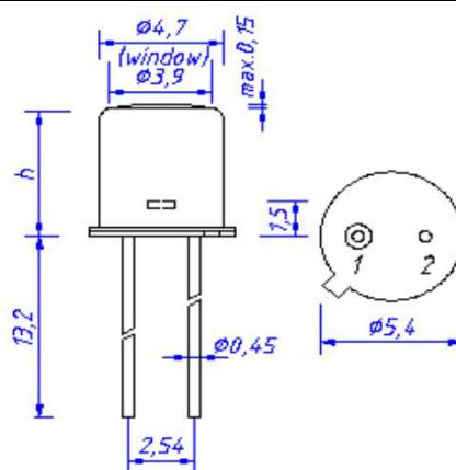
1 - anode, 2 - cathode + case, h=3.7 mm
