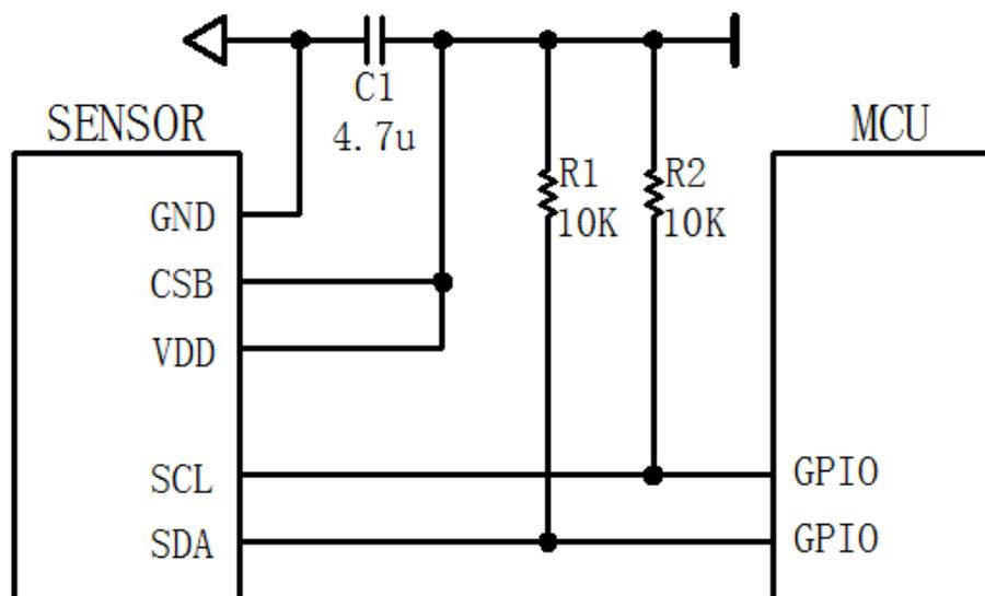
Figure3: Typical application circuit
