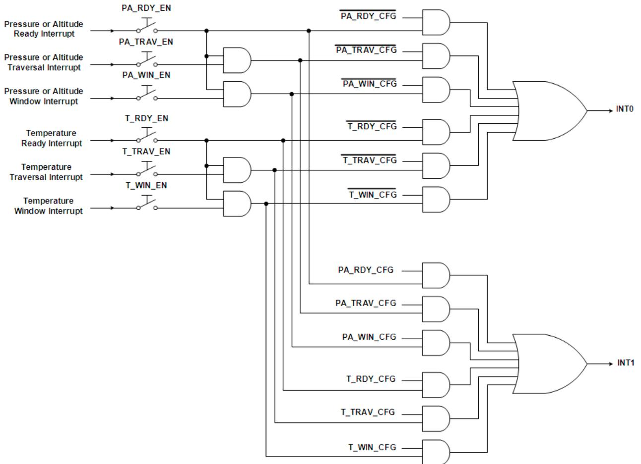
Figure 2: Interrupts mapping diagram
