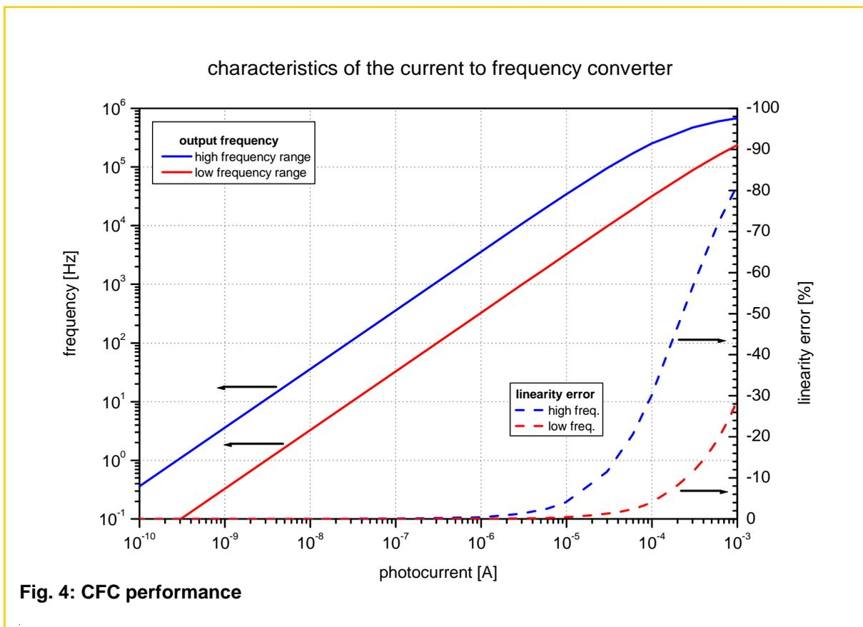
**Hint:** If you require different conversion factors the load capacitors CL1 and CL2 have to be changed. CL1 is solely active with switch 1 opened. Closing switch 1 puts both capacitors in parallel and the active load capacitance equals their sum. We are happy to assist you with that or to deliver boards adapted to your application.
