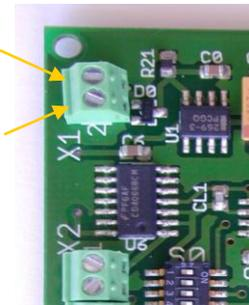
Fig. 2: Power supply connection
