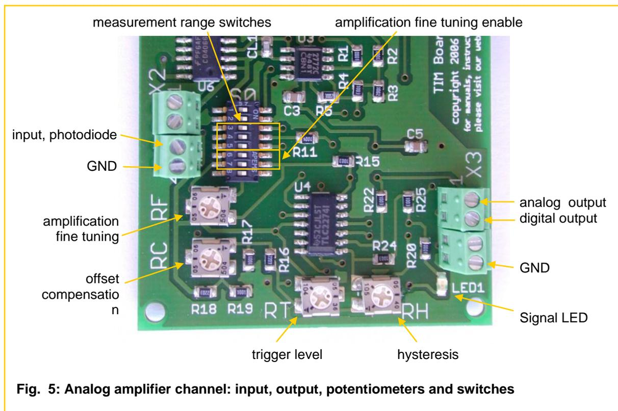
**Fig. 5: Analog amplifier channel: input, output, potentiometers and switches**
