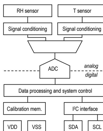
Figure 1 Functional block diagram of the SHTW2.
