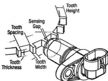
For best results, we recommend targets made from low carbon cold rolled steel. Other factors that influence sensor performance include gear tooth height and width, space between the teeth, shape of the teeth and thickness of the target. As a general guideline, consider a target with minimum parameters as shown below. Note that smaller dimensions may work, but testing for the application is required.
