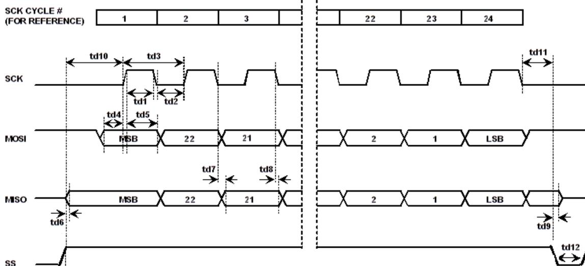
Figure 2: SPI Timing
