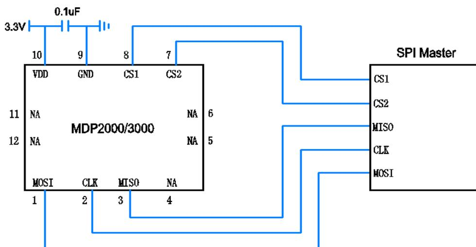
Note: the capacitors should be placed as close as possible to the VDD pin
