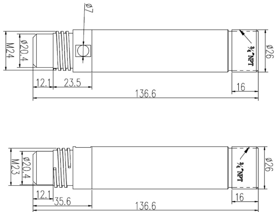
Figure 2: Sensor dimensions
