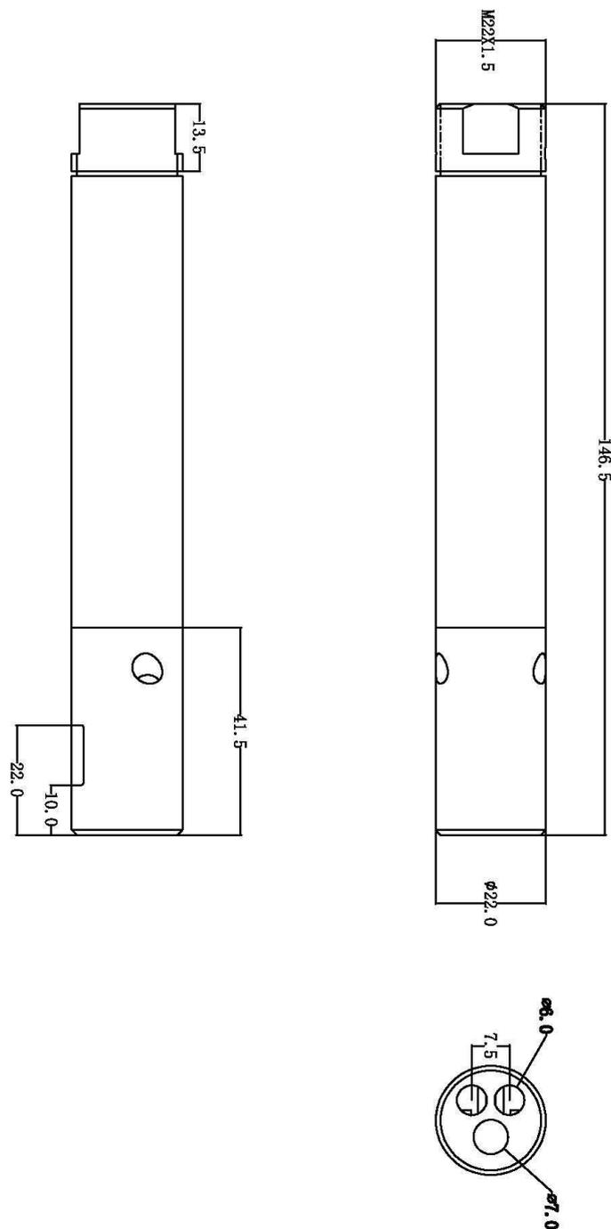
Figure 2: Sensor dimensions
