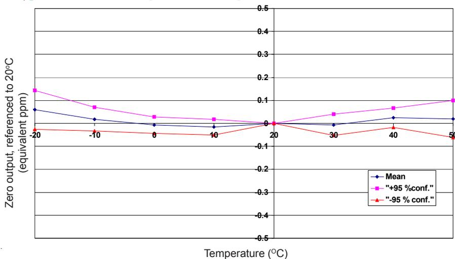
Figure 3 shows the variation in zero output caused by changes in temperature, expressed as ppm gas equivalent.
