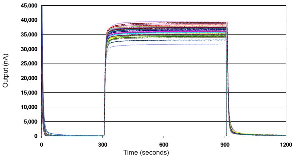
Figure 4 shows the response to 400ppm H<sub>2</sub>S for 64 sensors. Repeatable zero, fast response and stable output are the result of good process control.
