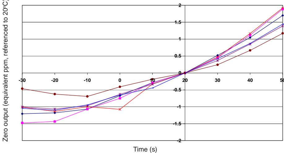
Figure 3 shows the variation in zero output caused by changes in temperature, expressed as ppm gas equivalent, referenced to zero at 20°C.
