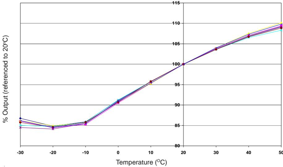
Figure 2 shows the variation of sensitivity due to changes in temperature.
