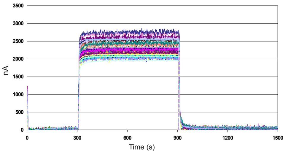
Typical batch of 64 sensors all respond rapidly and repeatably to 10ppm SO<sub>2</sub>.
