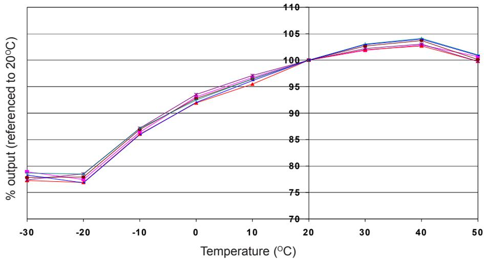
Figure 2 shows the variation in sensitivity caused by changes in temperature. This data is taken from a typical batch of sensors.
