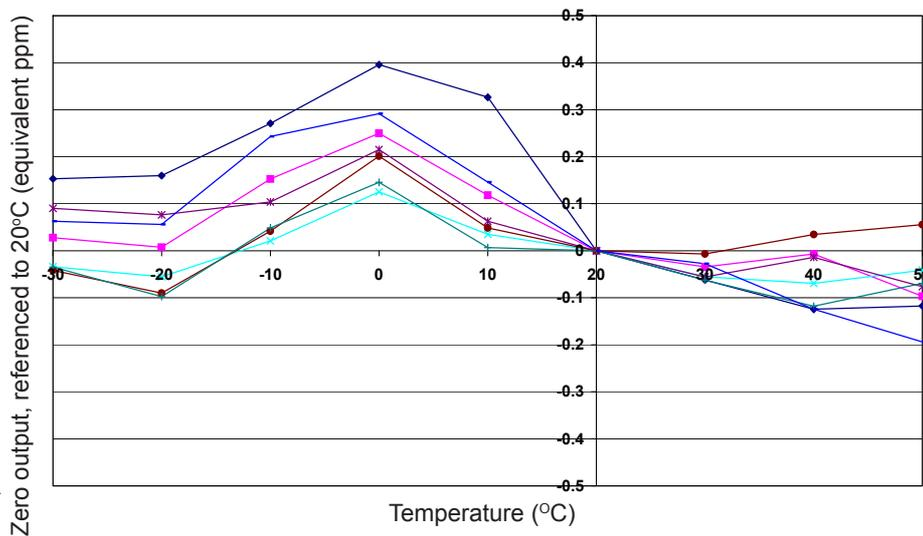
Figure 3 shows the variation in zero output caused by changes in temperature, expressed as ppm gas equivalent, referenced to zero at 20°C. This data is taken from a typical batch of sensors.
