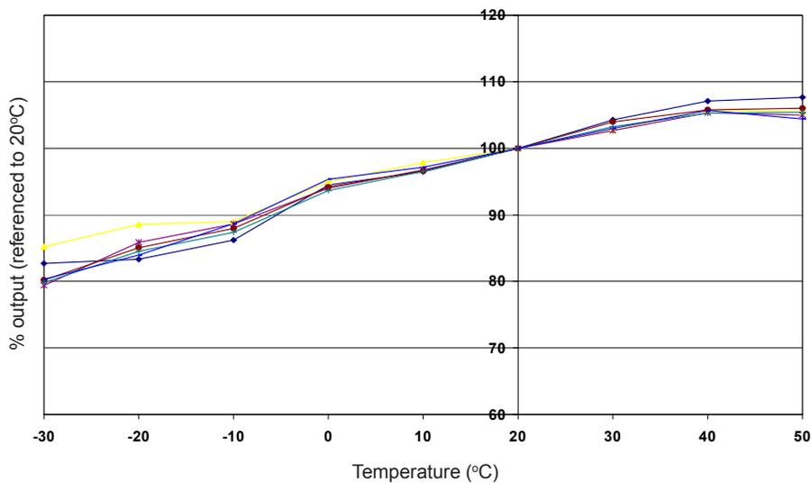
Figure 5 shows the variation in sensitivity caused by changes in temperature.
