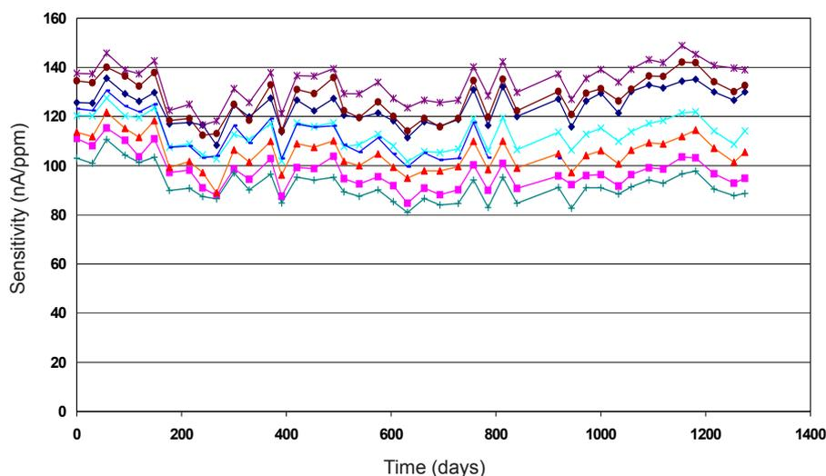
Figure 7 shows good long term stability to H<sub>2</sub>S for the D2 sensor.
