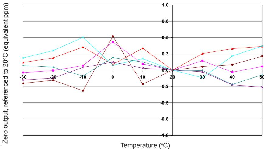
Figure 6 shows the variation in zero output caused by changes in temperature, expressed as ppm gas equivalent referenced to 20°C.
