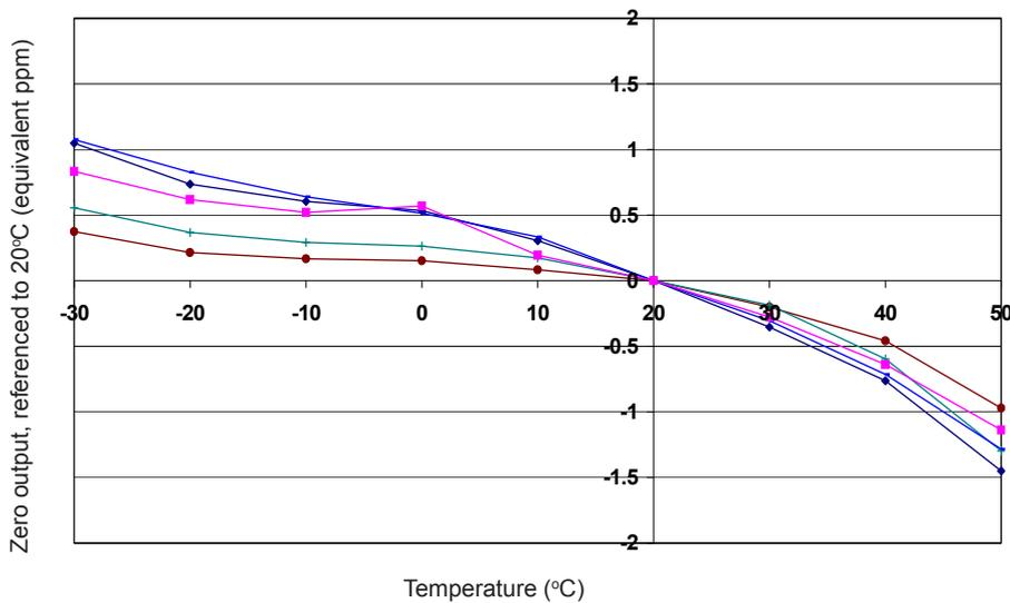
Figure 3 shows the variation in zero output caused by changes in temperature, expressed as ppm gas equivalent referenced to the zero at 20°C.
