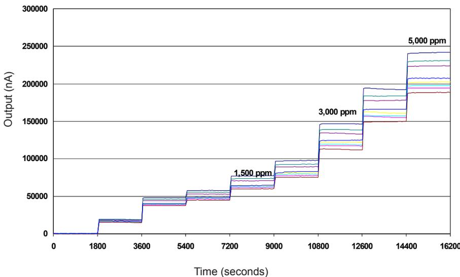
Figure 4 shows the response for a batch of D2 sensors tested with CO gas up to 5000ppm. The fast, stable response shows a robust sensor that operates well above its specification.
