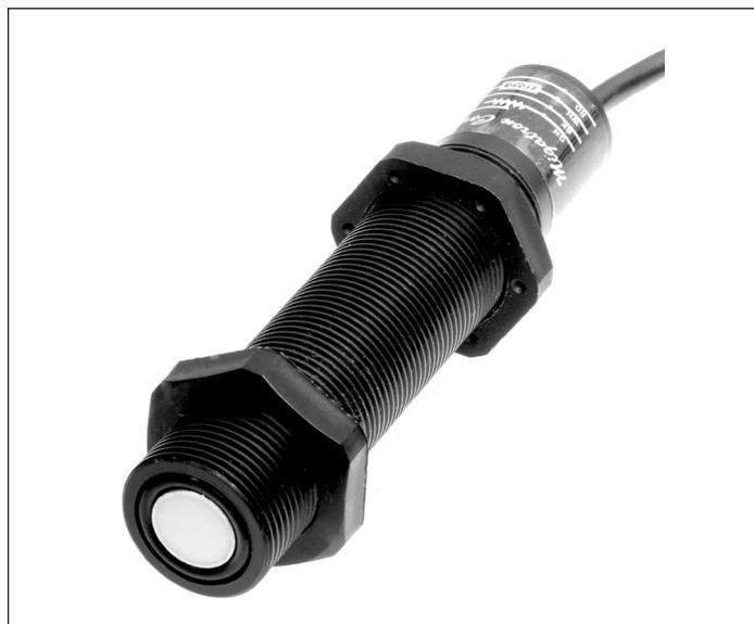
between the green lead and black lead of the cable the maximum range can be set from 5 to 30 inches. The resistor chart on the following page provides resistance values and the approximate resulting sensing range. These sensors provide precise proximity or level sensing regardless of color, density or transparency. They are equally effective on liquid, metal, plastic and glass targets. A standard 6 foot cable is provided. Call factory for optional cable lengths.
