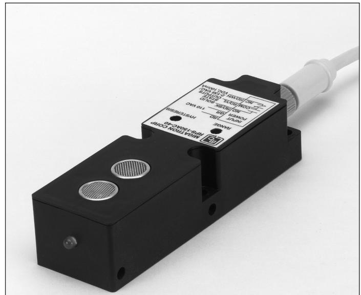
Yellow indicates a weak signal and bright red indicates a strong signal. The frequency of operation is 38.5kHz. There are two ranges available in this model 2 - 40" or 5 - 80". It also features a quick disconnect (QD) receptacle. The housing is constructed of PBT plastic and has standard 30mm x 60mm limit switch mounting dimensions as well as side holes for mounting the sensor on its side.
