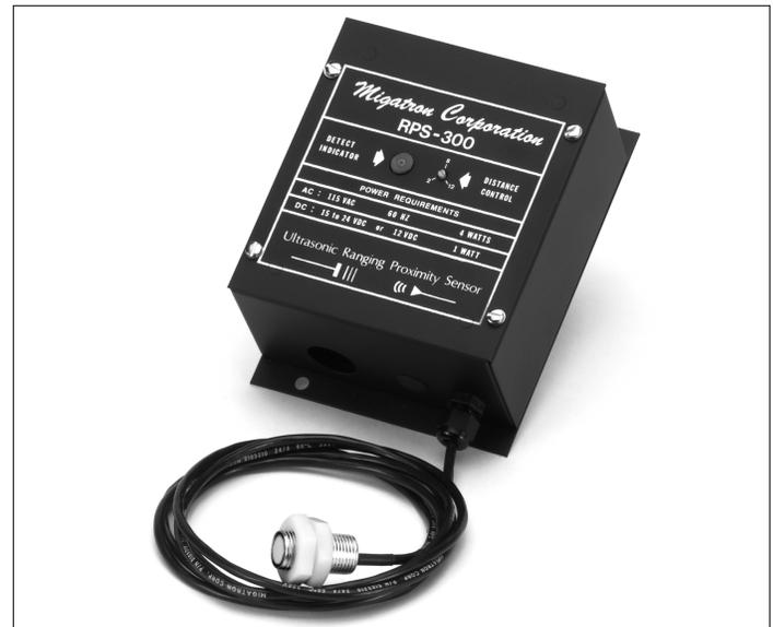
are supplied. The RPS-300 sensor operates at a frequency of 222kHz for the 14" and 36" ranges and 150kHz for the 72" range. This sensor has a narrow sensing beam. Sensing ranges available for the RPS-300 include 4" to 14", 5" to 36", and 8" to 72". Mounting flanges, LED indicator, ranging potentiometer and 6-ft. transducer cable are included. Optional cable lengths are available.
