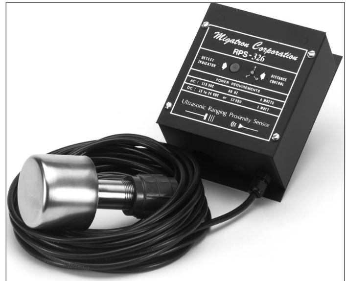
outputs are supplied. The RPS-326 sensor, which operates at a frequency of 37kHz, has a narrow sensing beam. Sensing ranges available for the RPS-326 include 24" to 72", and 24" to 240". Mounting flanges, LED indicator, ranging potentiometer and 30ft. transducer cable are included. Optional cable lengths are available.
