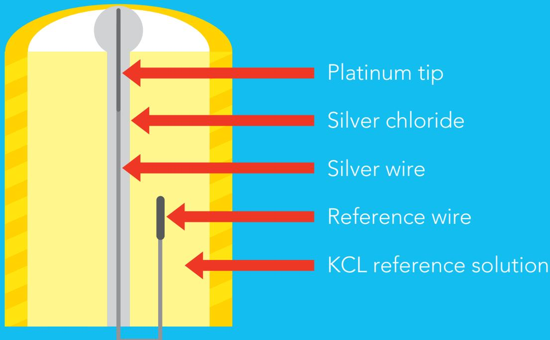
An ORP probe is a passive device that detects a current generated from the oxidation or reduction chemical substances in water. This current (which can be positive or negative) is very weak and cannot be detected with a multimeter, or an analog to digital converter.
