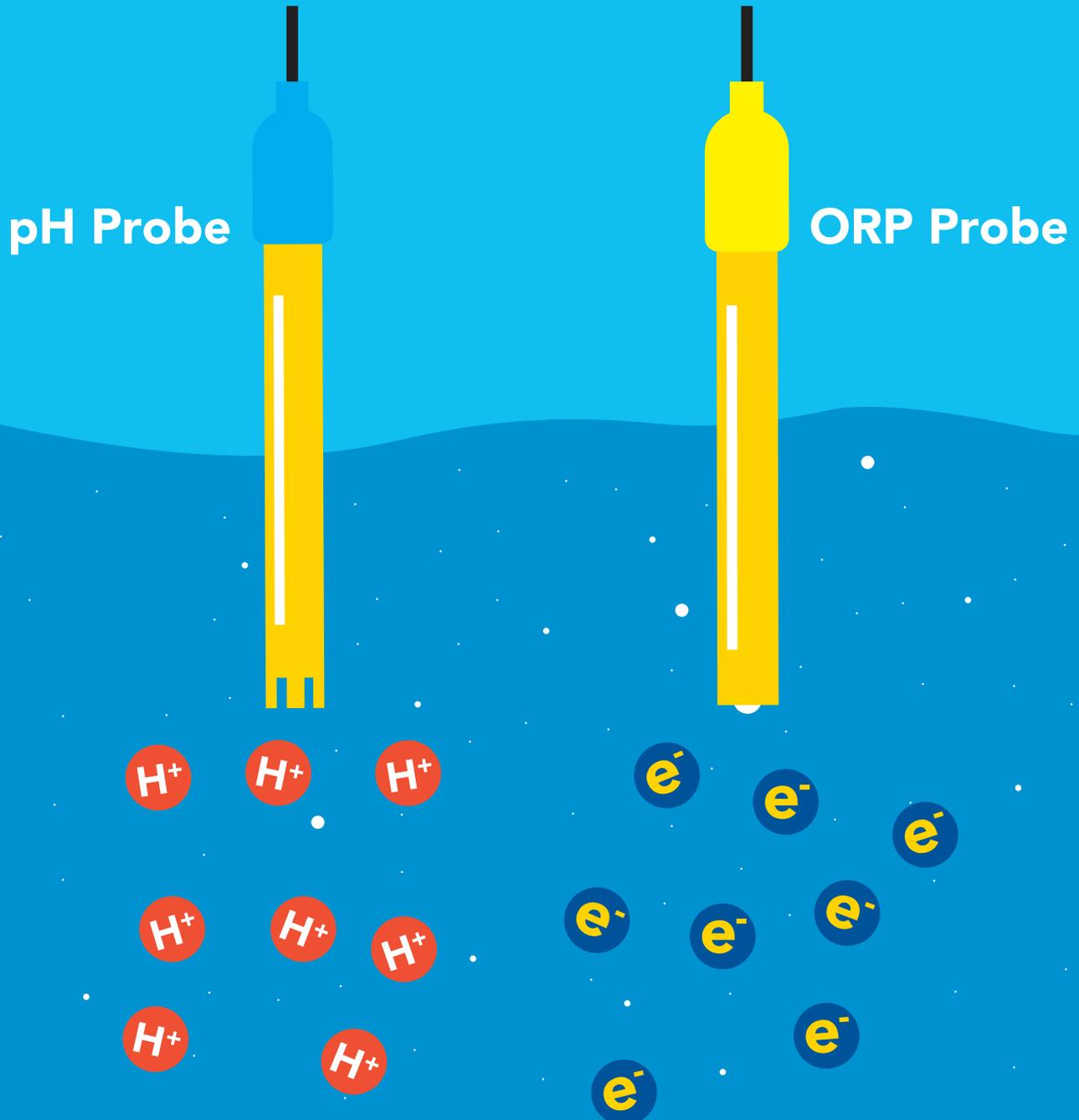
When reading the ORP of a liquid that has very few electronics available for transfer ORP readings can appear to be inconsistent.
