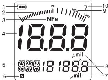
1. Battery power symbol, shows the battery power
