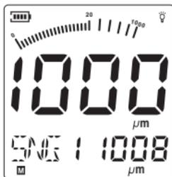
To ensure a precise two point calibration, repeat step b and c to improve measurement precision and reduce incidental error.
