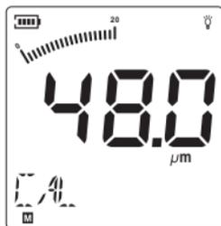
Press “▲” and “▼” key to adjust the display value to be equals with the standard piece's thickness, and then place the next standard piece on the iron basic to calibrate.
