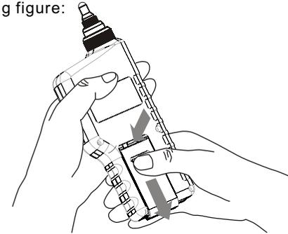
b. Insert a 9V battery into battery compartment, note the battery polarity, and then close the battery door, as shown in following figure:
