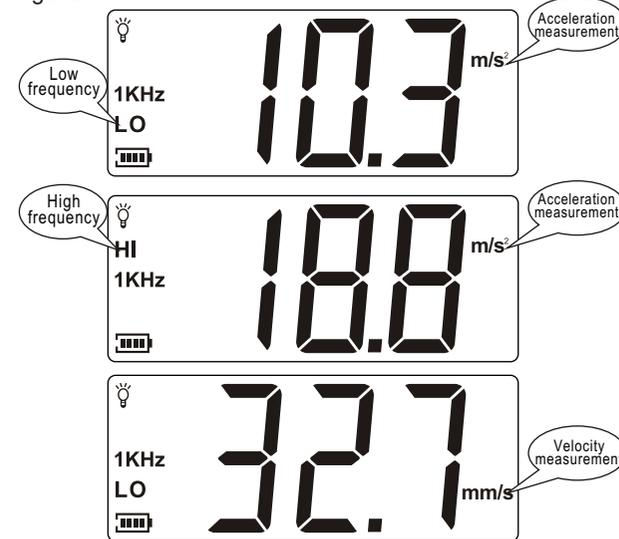
**Select High/low Frequency:( High frequency is only for acceleration measurement mode)**
