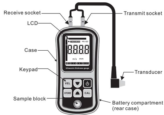
be cleaned for preventing rust. In higher temperature environment, be sure protect the block form the droplet of water. If the gauge is not use for a long period, please apply some antirust on the sample block.
