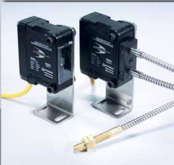
The **SMARTEYE® STEALTH-UV™** luminescent sensor detects fluorescent properties found in inks and additives that can be used for product inspection/verification on a wide variety of materials. Many materials have natural UV fluorescent properties that can also be detected, such as:
