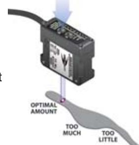
**D. Two-Point AUTOSET Mode** – Use this mode to establish upper and lower limits. When monitoring the target luminescence using the analog output, this mode will set your upper and lower control limits at specific points on the analog output scale. This is the most sensitive mode for detection of low contrast differences in two UV luminescent materials. An example would be glue on a white paper envelope, where both the glue and the paper have optical brighteners present.
