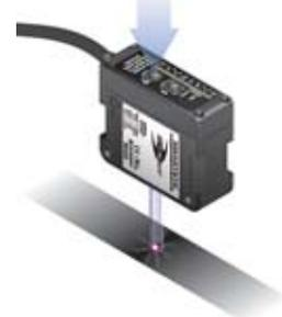
**C. Mid-Point AUTOSET Mode** – This mode is recommended for use in analog output applications only. With the luminescent material in view, the sensor samples the signal level from the target and sets the sensor at the switching threshold. The sensor's analog output then reflects the level of fluorescence as compared to the target...either higher or lower than the sampled signal level. This can be used as part of a feedback loop to maintain or control the flow of materials at an optimum level.
