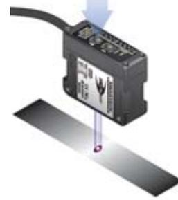
**B. Dark State AUTOSET Mode** – With background in view, the sensor samples the signal level from the background and sets the switching threshold just above that signal level. The sensor is sensitive to more luminescent materials in this mode. This mode is useful in solving many common applications. The analog output can be used to provide feedback of target brightness level for control applications in this mode as well.
