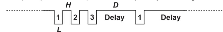
Each pulse (L) is low for 40ms to 400ms. The idle time (H) between pulses is 40ms to 400ms. The delay (D) between sets of pulses is .75 seconds to 5 seconds.
