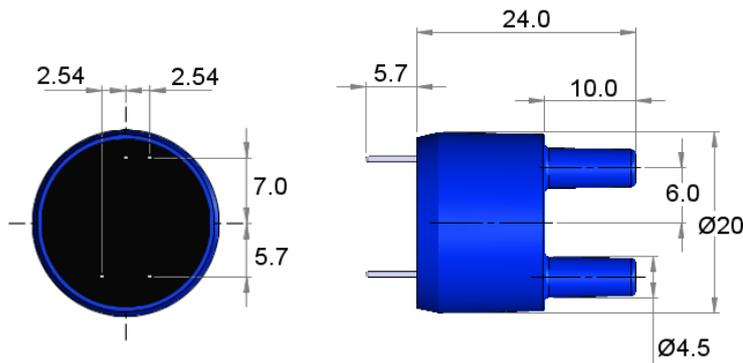
**NOTE:** 4.5mm OD push-fit tubing connectors.
