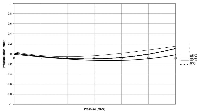
Temperature Error Accuracy vs temperature (typical)
