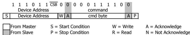
Figure 10: I<sup>2</sup>C Reset Command
