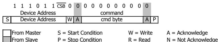
Figure 14: I<sup>2</sup>C ADC read sequence
