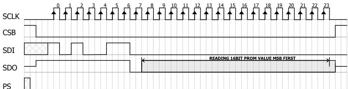
Figure 9: PROM Read sequence, address = 011 (Coefficient 3).
