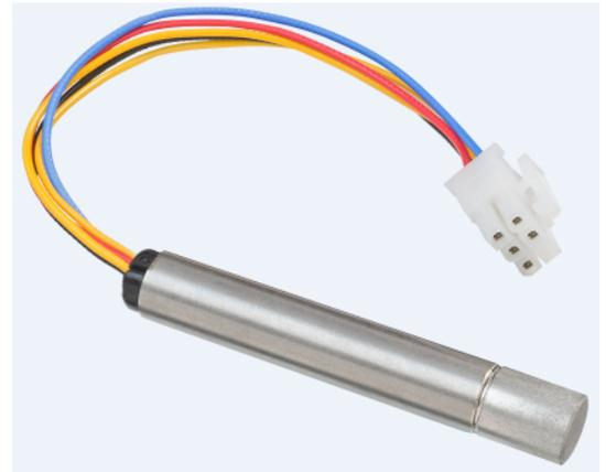
A heat element produces the 700 °C [1292 °F] required for the  $ZrO_2$  to operate as an  $O_2$  pump. The time taken for the pump to achieve specific minimum and maximum pressures within this chamber is a measure of the partial oxygen pressure of the environment.
