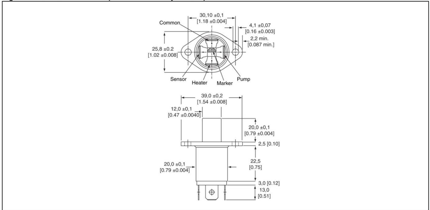
Figure 2. KGZ-10SP Dimensions (For reference only: mm/in.)
