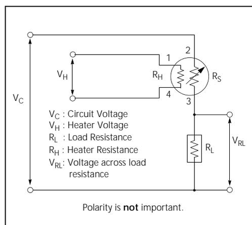
Fig 2. Standard circuit
