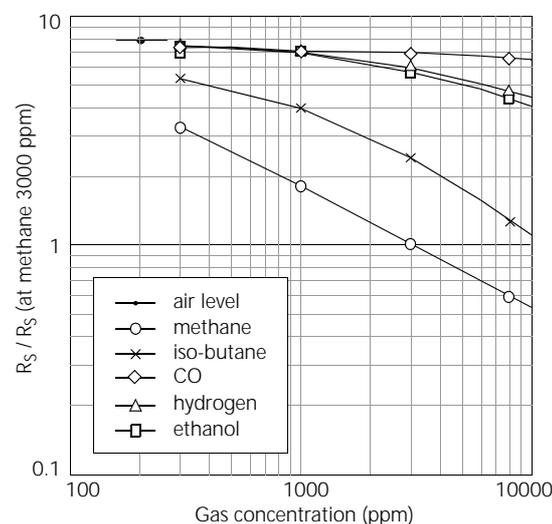
Fig 3. Sensitivity characteristics
