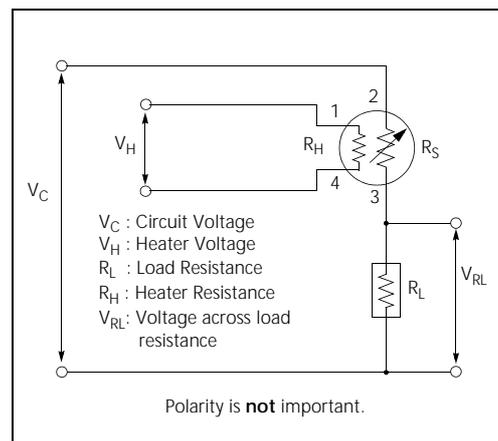
Fig 2. Standard circuit
