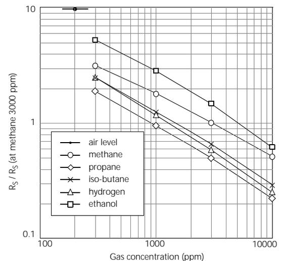
Fig 3. Sensitivity characteristics
